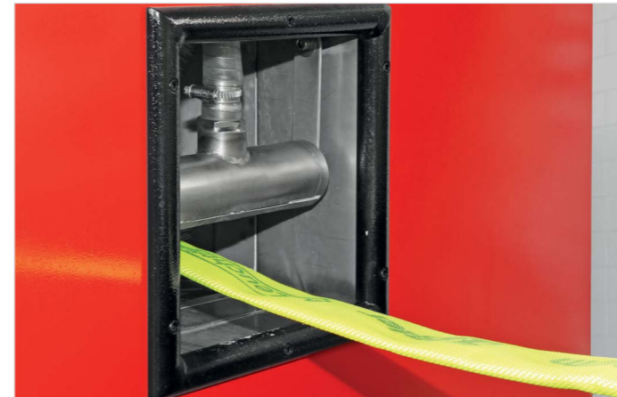
Parallel to this working step the cleaned hose is pre-dried by air. The moisture is blown off the hose.
