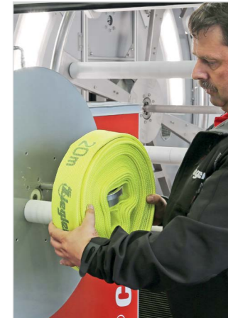
The wound hose: quickly cleaned, checked, absolutely dry and ready to use or to store.
