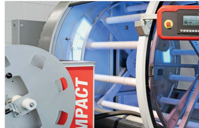
Start of the washing process: The hose is cleaned automatically with the help of brushes and high-pressure. This working step is indicated by blue light.
