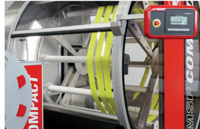
The hose will be rolled on the test drum before the testing-process finally starts.
