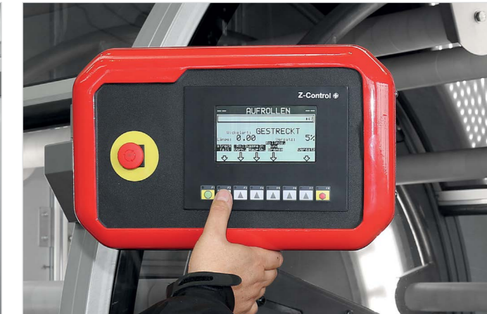
On the control panel the user can choose between single or double wound hoses.
