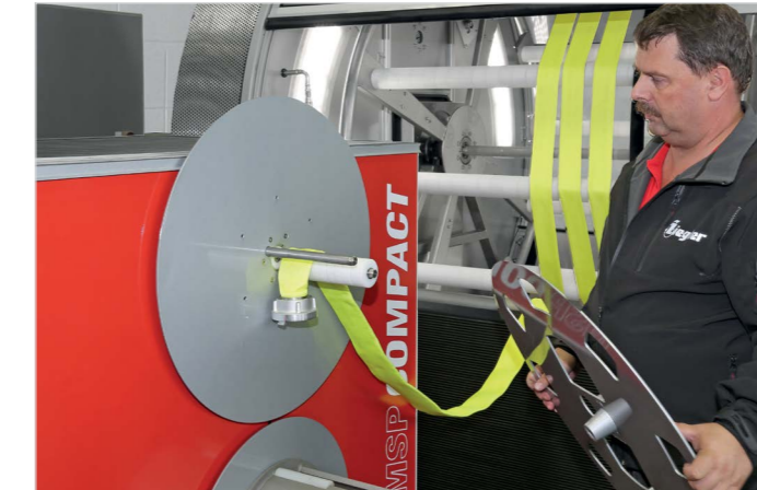
To prepare the hose-winding the hose needs to get hooked on the winder. The winder-disc is placed for safety.
