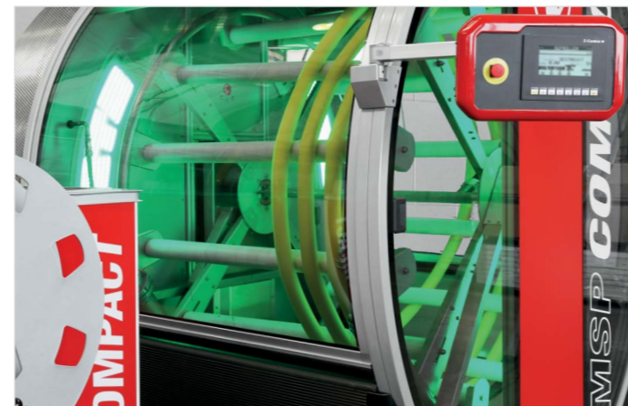
To dry the hose it will be constantly perfused with warm water. The moisture on the hose surface vaporizes by using the energy stored in the hot water. During the drying process LED lights will be shown.
