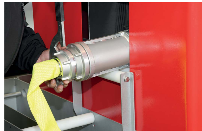
An adapter will be connected with the hose and pulls the hose, which needs to be cleaned, through the washing unit.
