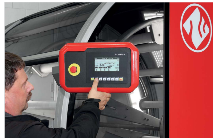
All operations are initiated via the Z-Control panel.
