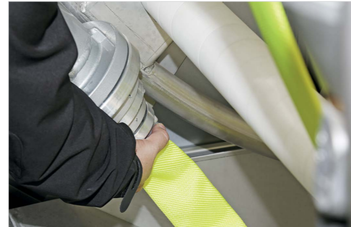
For preparing the testing and drying working step the hose will be coupled to the charging station.
