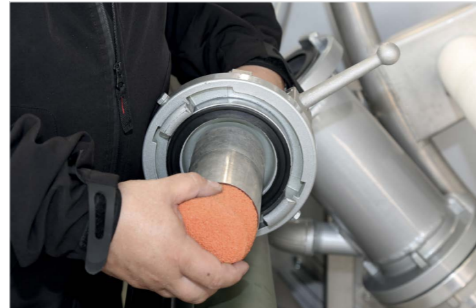
For inside-cleaning and drying of the hoses, the machine is equipped with a cleaning sponge.
